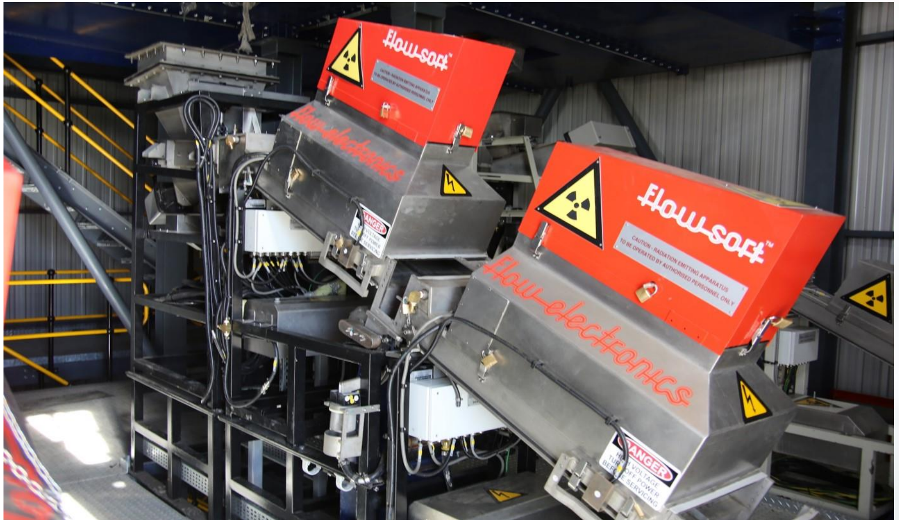
X-ray Flowsort machines in the New Recovery Building prior to commissioning. Used to extract diamonds from the dense DMS concentrate
