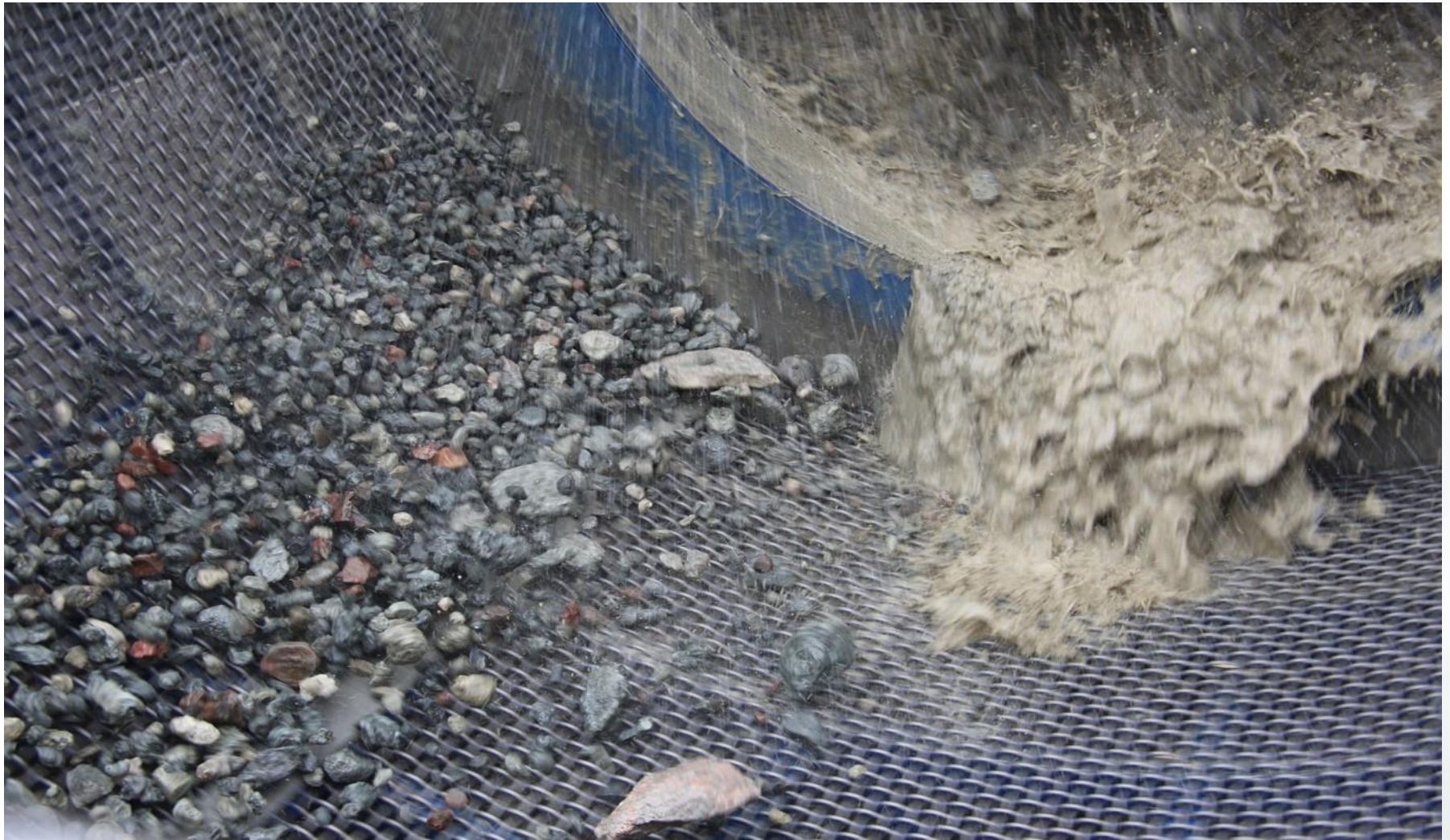
Kimberlite Ore passing through the new Primary Scrubber and Trommel
