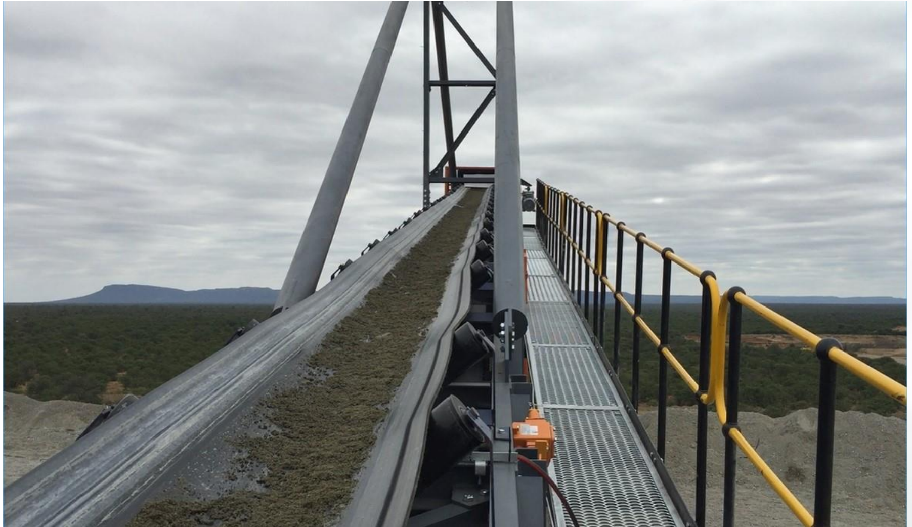
Barren Kimberlite rock from the DMS being conveyed to the Coarse Tailings Dump
