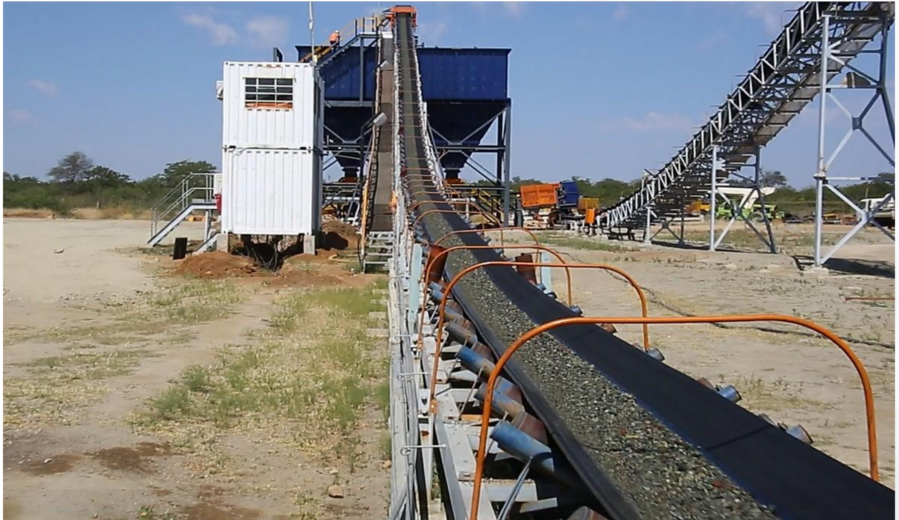
Scrubbed and Screened Ore being conveyed to the 400 tonne bin prior to being fed into the DMS (Dense Medium Separator)
