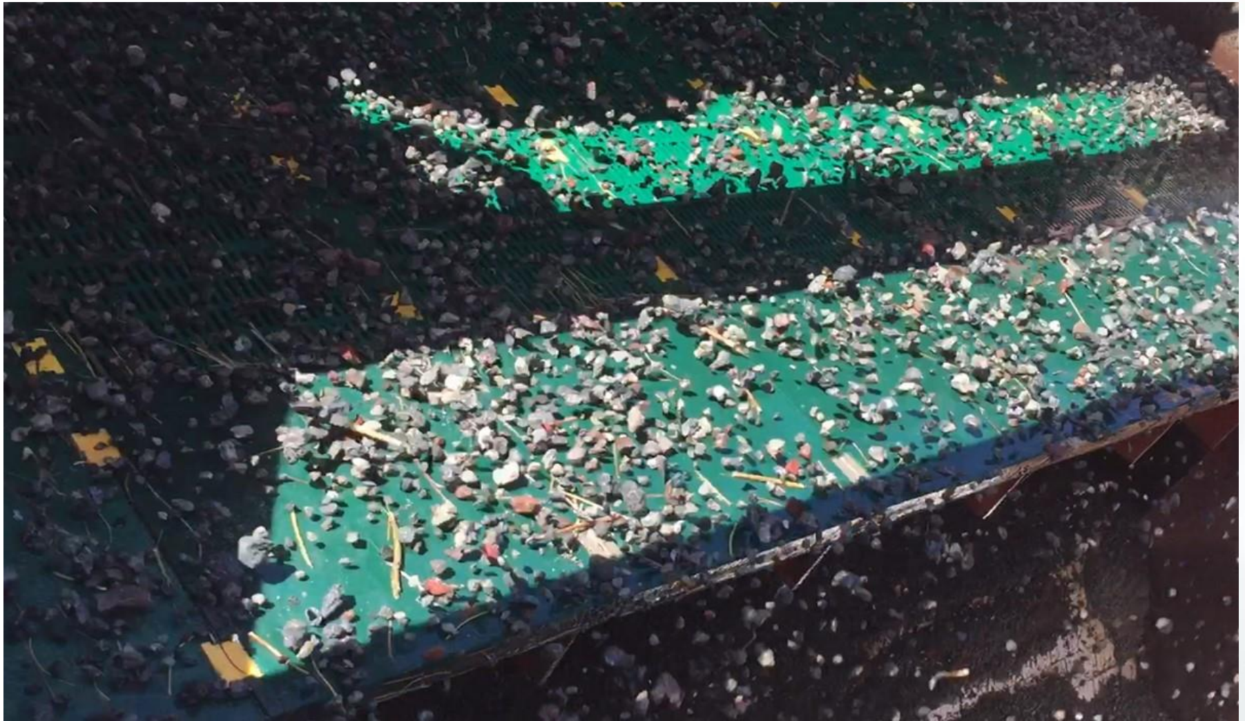
Kimberlite Ore passing over Sizing Panels in the Vibrating Secondary Screen
