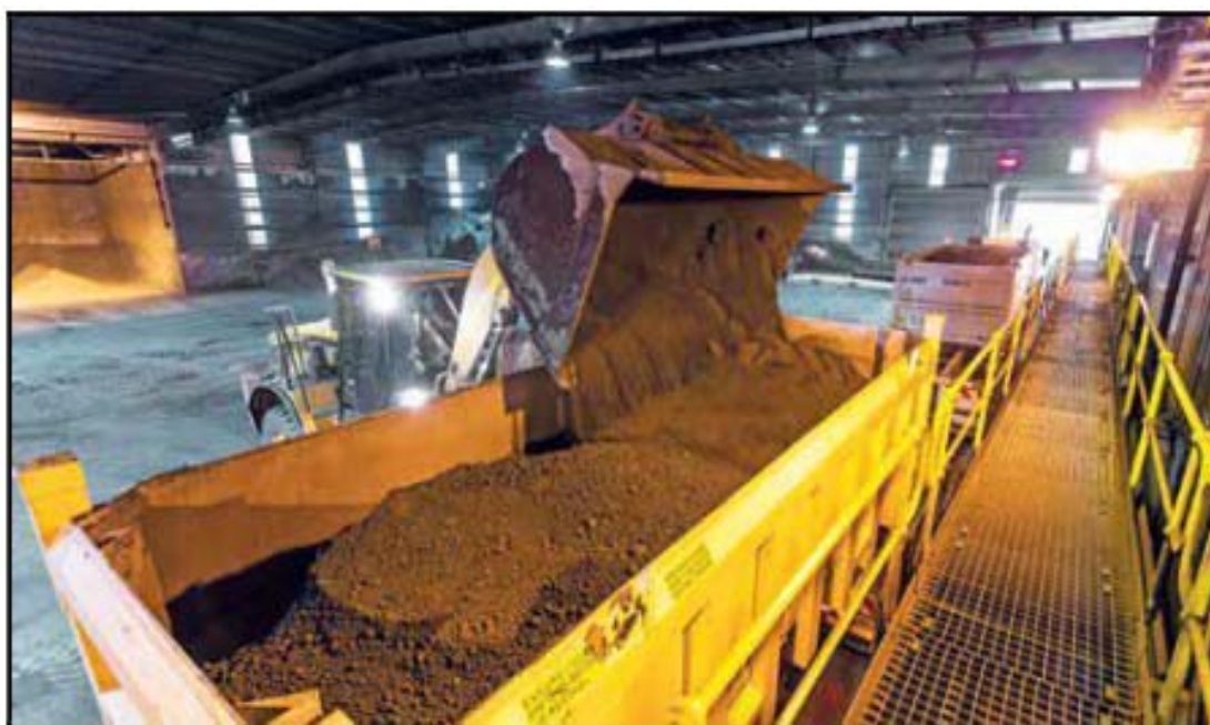
Figure 9 – Loading of a Rotabox (Source: Qube)
