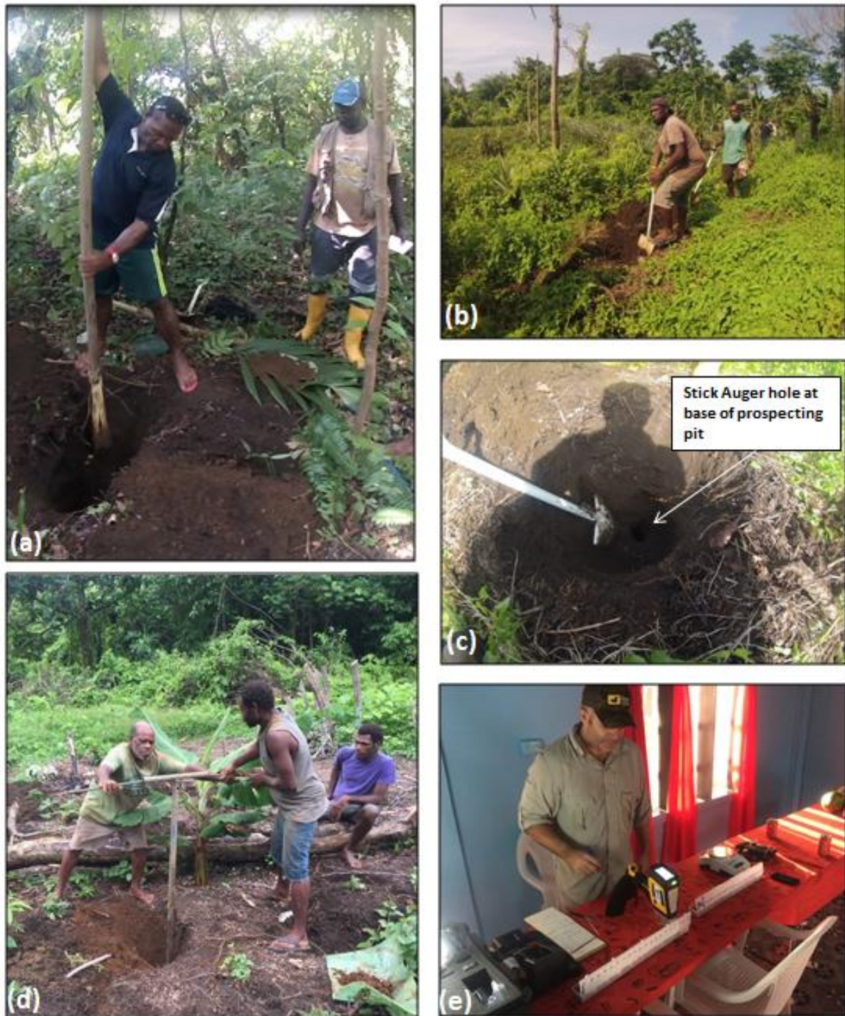
Figure 4: (a) Stick Auger being used for sampling bauxite profile. (b) Land Owner assisting prospecting on his own farm. (c) Stick Auger hole at bottom of hand dug prospecting pit. (d) Conventional Hand-Auger sampling. (e) Field analysis using hand-held XRF.
