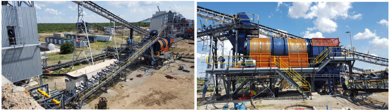
The new primary scrubber module with electrics in progress
