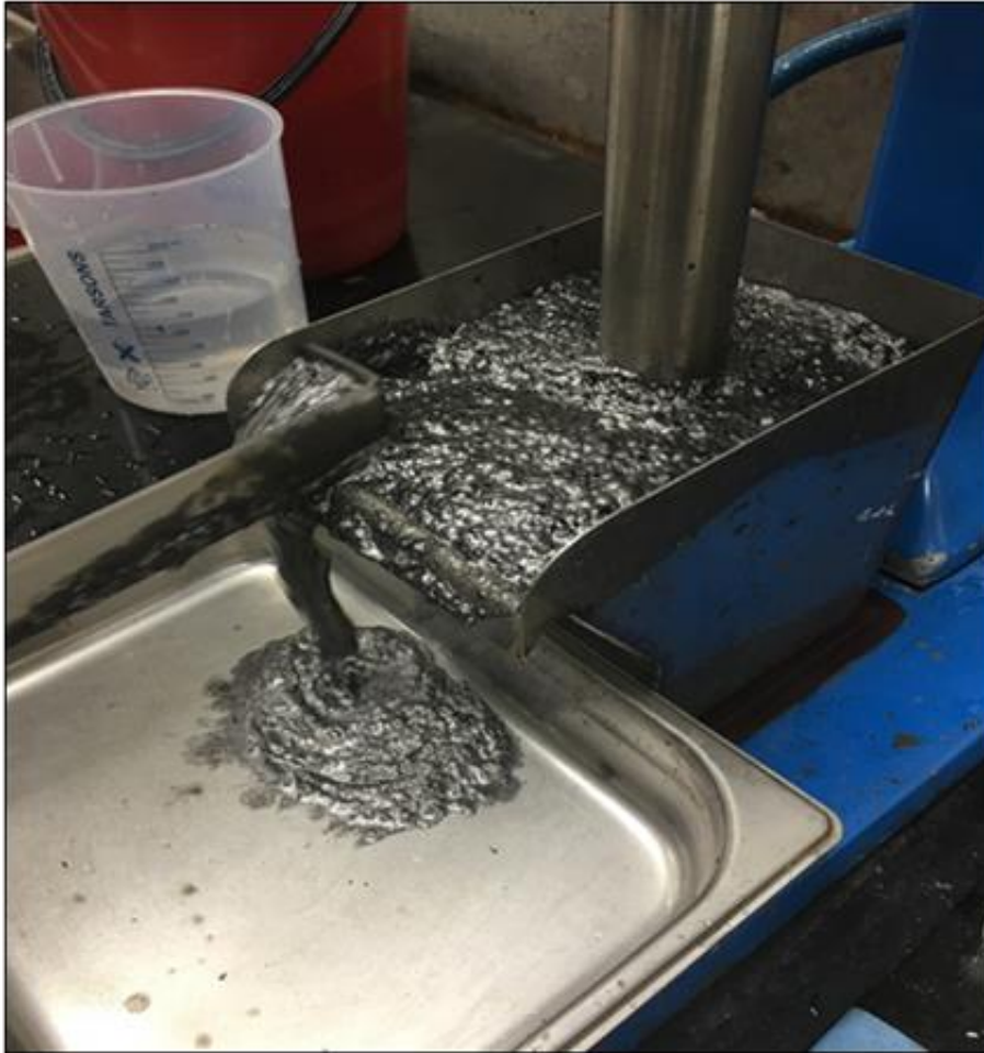
Figure 1. Laboratory cleaner flotation from the Company's graphite at the Elephant Deposit
