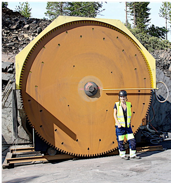
Figure 3. Dual blade diamond saw to commence trial graphite ore block cutting.
