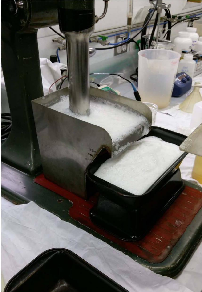
Figure 3 – Rougher Flotation Test On Lake Wells Derived Mixed Sulphate Salts.
