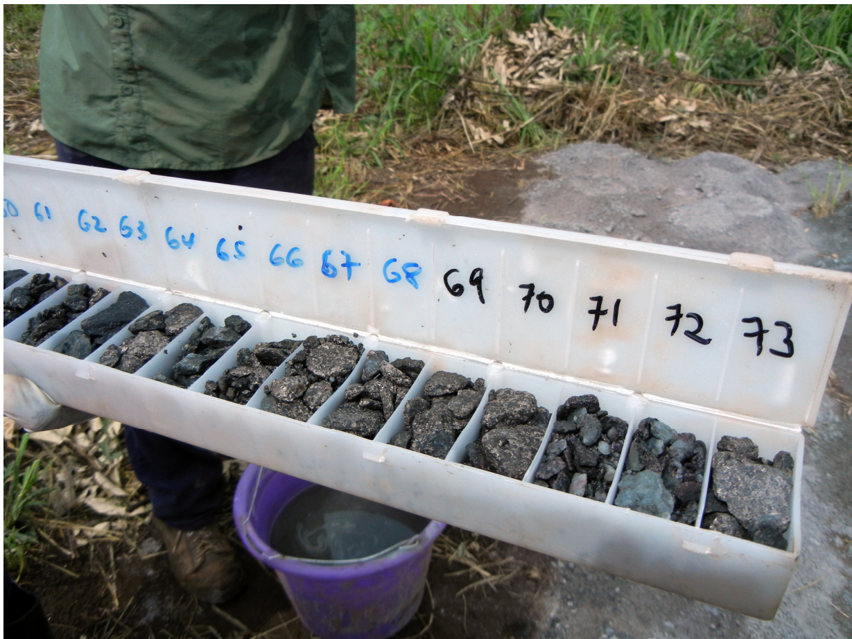
Image of AKC004 drill chips with strong matrix to massive sulphides from 63 to 73m
