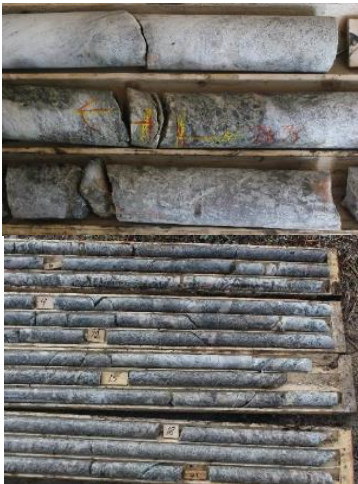
Figure 9. Drill Core from the Root Lake project showing multiple intersection of Spodumene mineralisation in the pegmatite structures.
