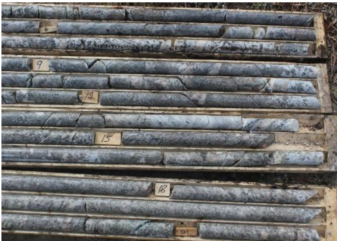
Figure 10. Drill core from the Root Lake Project showing multiple intersections of spodumene mineralisation in the pegmatite structures.
