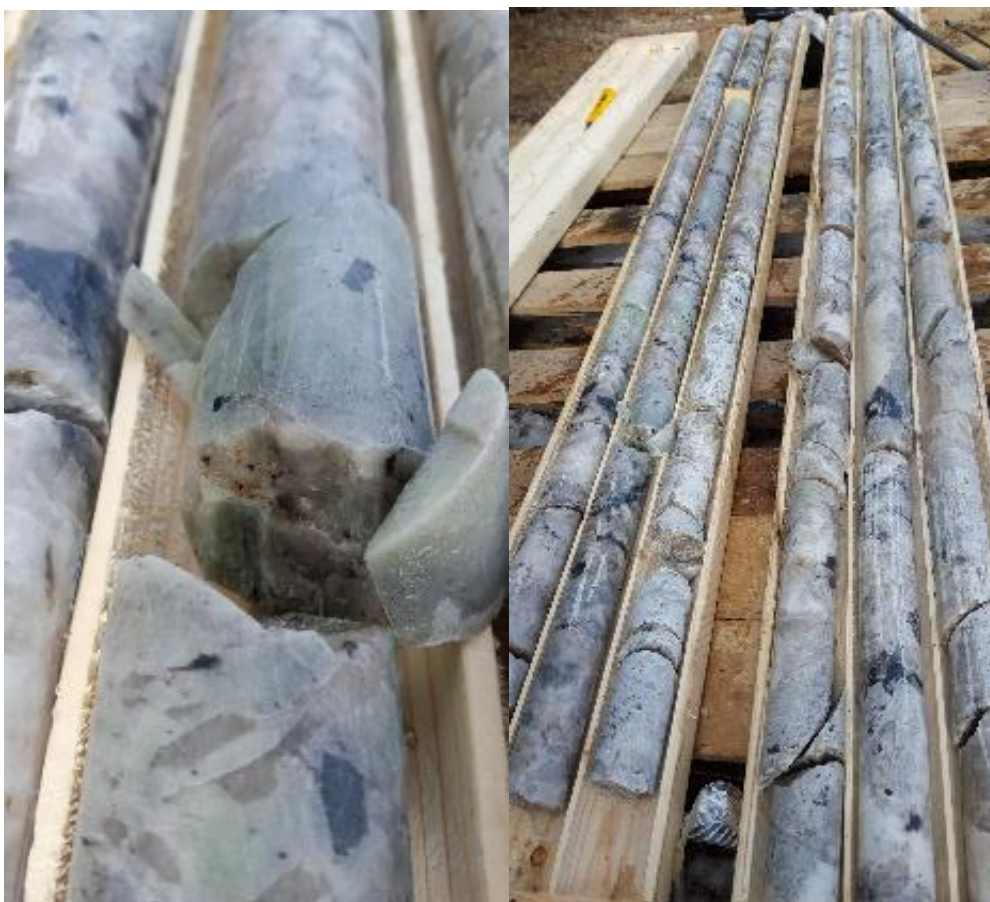
Figure 5. Drill core from the Seymour Lake Project showing multiple intersections of spodumene mineralisation in the pegmatite structures.
