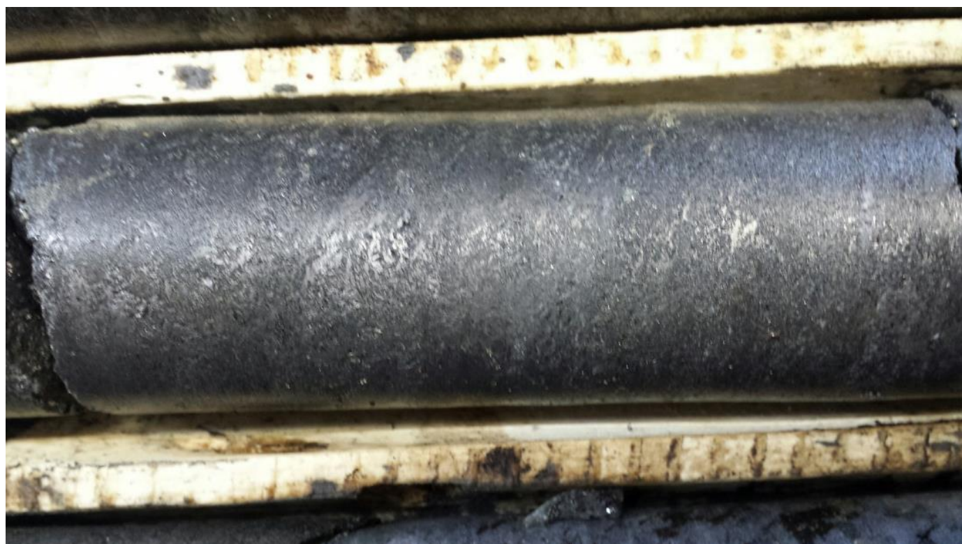
Figure 15. Graphite core from current drilling at Manitowadge graphite project in Ontario, Canada (Hole EM 12-05 at Silver Star Prospect)
