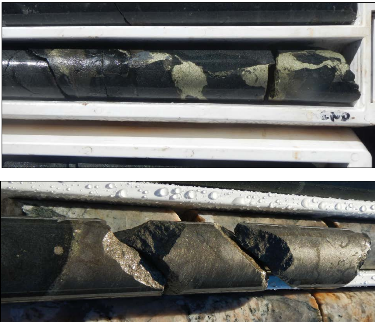
Figure 3 – photograph of drill core from MAD22 (top) and MAD23 (lower). MAD22 core shows chalcopyrite-rich stringer sulphides from 52-52.5m. MAD23 core shows massive nickel-copper sulphides from 57.45-57.7m that average 2.3%Ni, 5.1%Cu (based on field XRF analysis).
