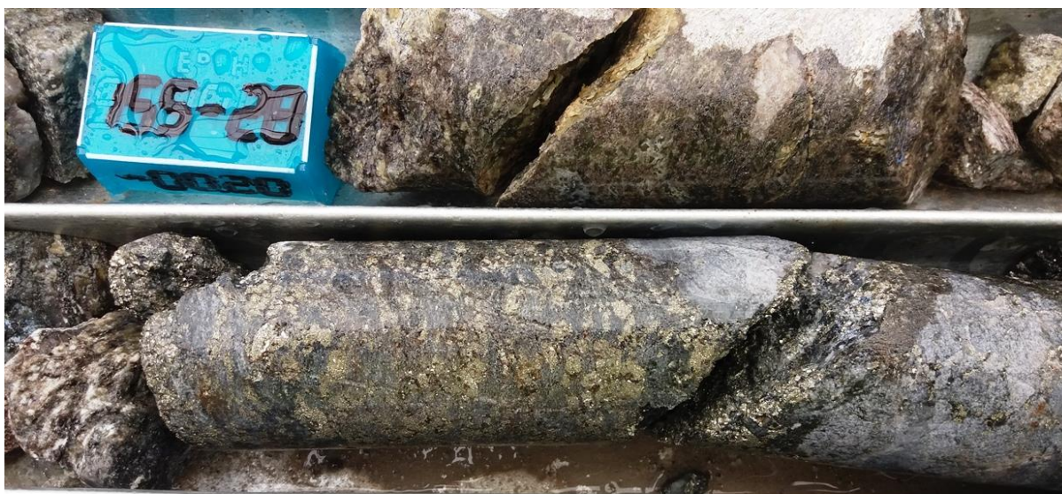
Figure 3: Massive sulphides in OCOD035 (157.8m down-hole, approximately 80m below surface) at the PC Project.
