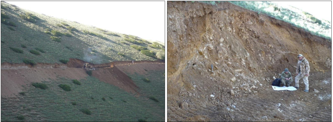
Figure 3 New mineralised shear zone (yellowish area) identified in bulldozer cutting 1 containing 2 metres a 9 g/t within a wide alteration halo
