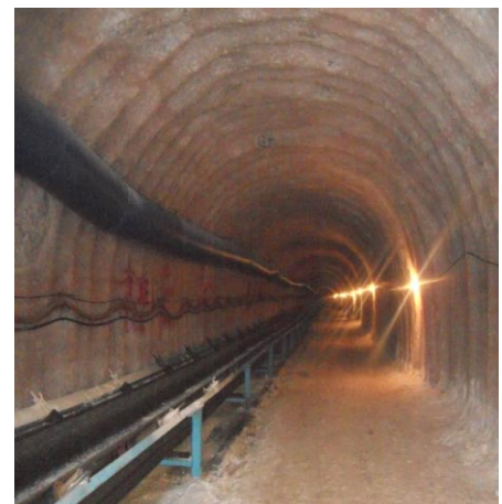
Thong Mang Potash Mine - underground production drive and conveyor belt
