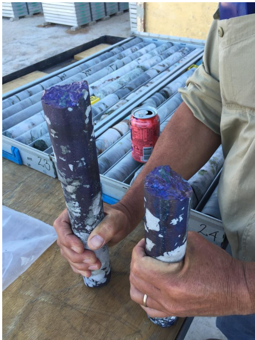
Figure 8: High-grade vein hosted copper sulphides (bornite) in drill core from T3 resource area
