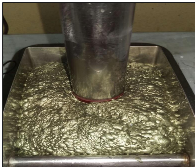
Figure 4: T3 Chalcopyrite flotation during test work
