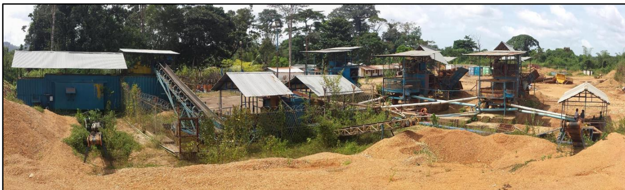
Photograph 1. View of recently purchased second-hand rotary pan plant, Kono District. The plant has since been dis-assembled and relocated to Sumbuya, EL 12/2014.
