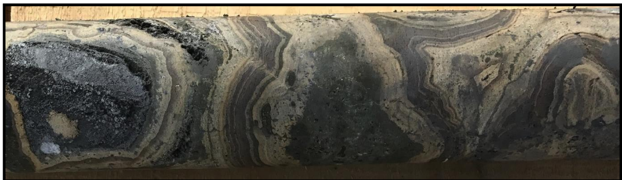
Figure 2: Massive colloform sphalerite (ZnS) breccia in drill core at Kildare (ZC16-001). Actual length 15cm.
