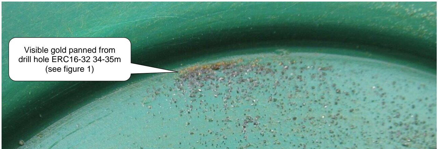
Figure 2: Fine grained gold extracted from drill hole rock chip samples 34-35 metre interval (figure 1). Drill assay was 41.6 g/t gold within 3 metres at 14.3 g/t gold
