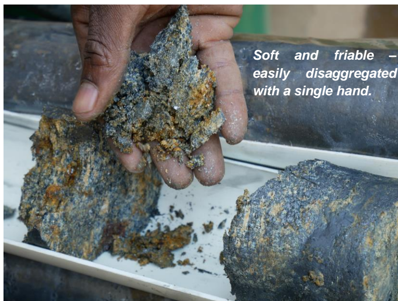
Figure 1. Typical high-grade, saprolite-hosted flake graphite MGDD0004: 22.5m downhole.
