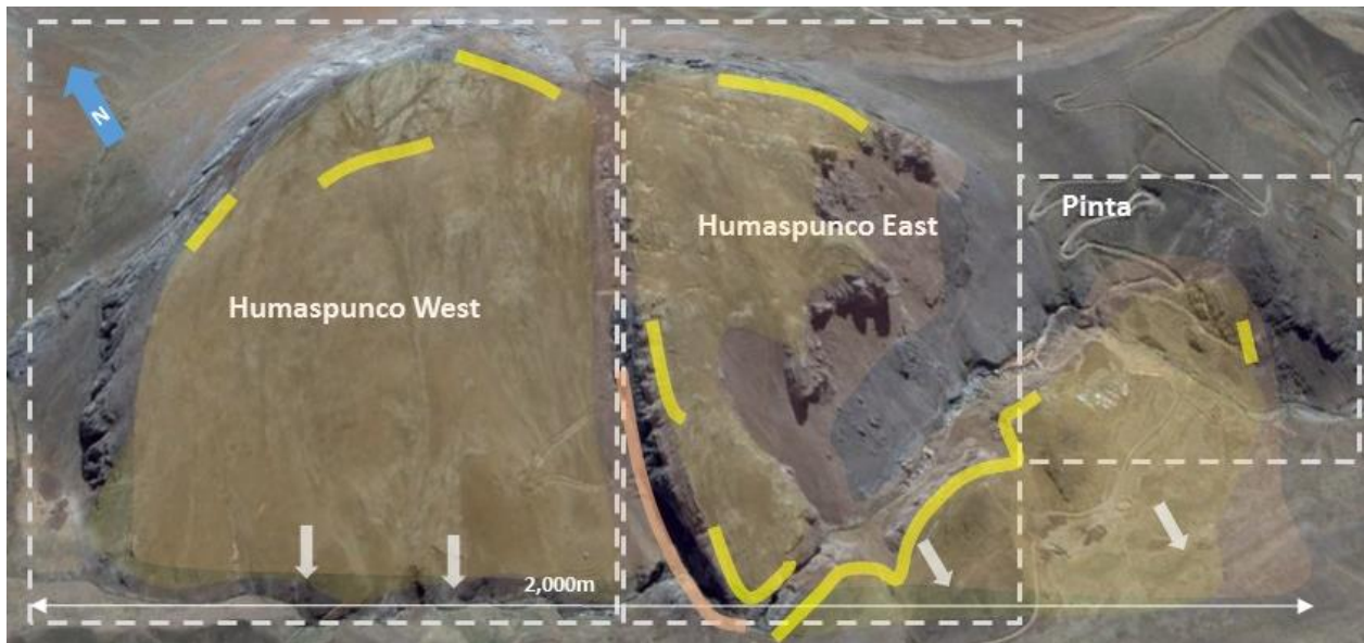
Figure 6 ABOVE: Satellite image showing Humaspunco and Pinto Prospects. Pale yellow shading shows the projected expanse of the upper manto sequence, connecting outcrop occurrences of three manto horizons (thick yellow lines). The pale beige shading shows the projected expanse of the lower manto sequence, connecting outcrop occurrences of a fourth manto horizon (thick beige lines).
