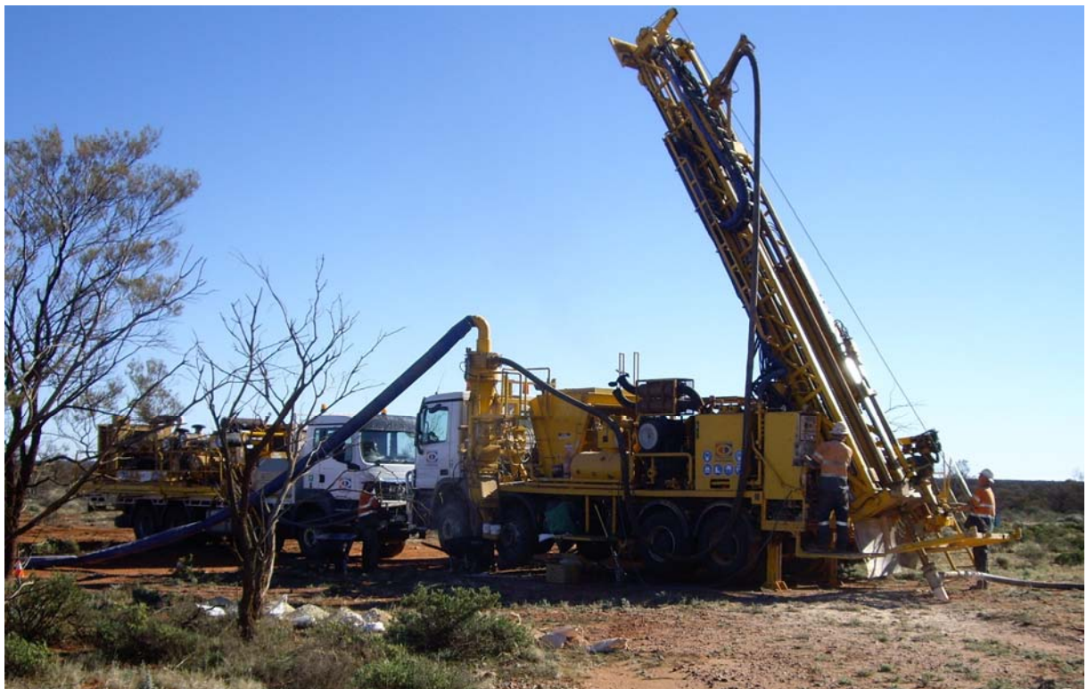
Picture 1.2.1: Slimline RC Drilling in the Challenger Matrix
