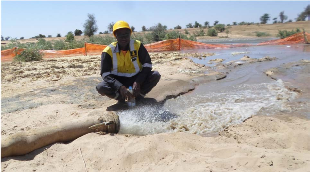
Figure 5: BAUER Resources Senegal water airlift testing at Process Water Bore 1
