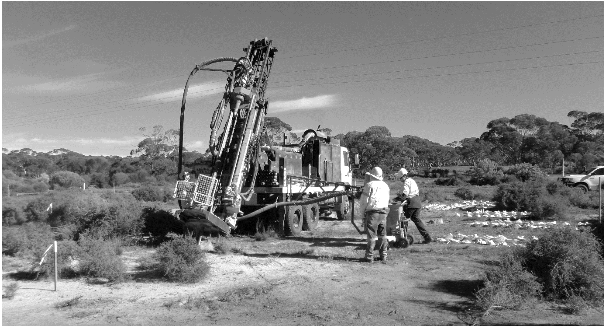
Photo: Aircore drilling at Burbanks North, August 2016 (Copyright: G. Harvey)
