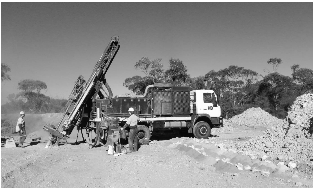
Photo: RC drilling at Newminster, April 2016 (Copyright: G. Harvey)
