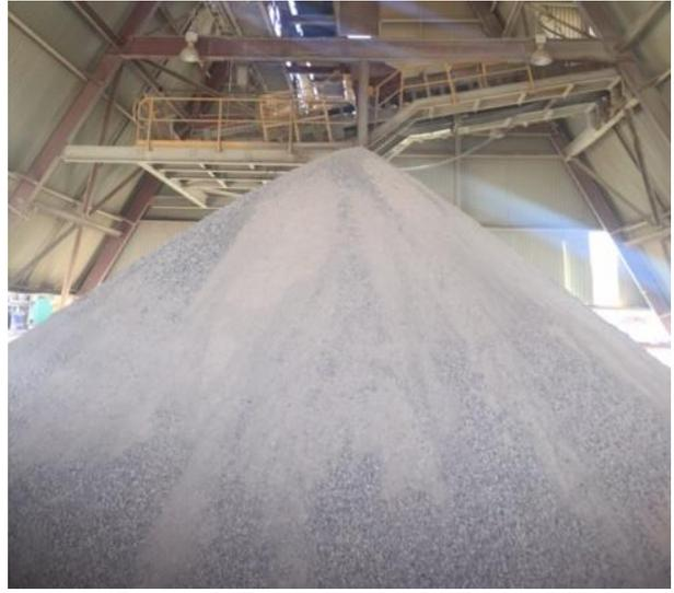
**Photo 4: Fine ore shed filling with ore**
