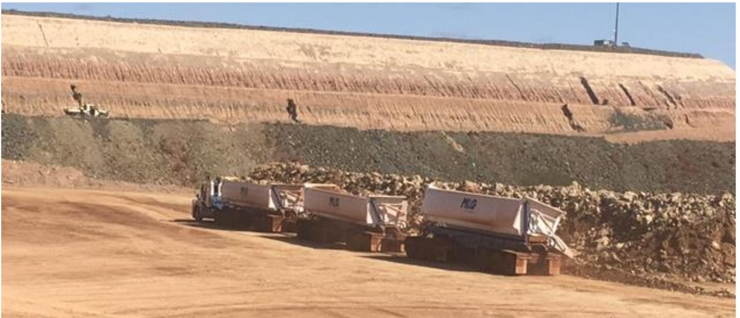
**Photo 2: One of two MLG road trains hauling ore back to ROM**
