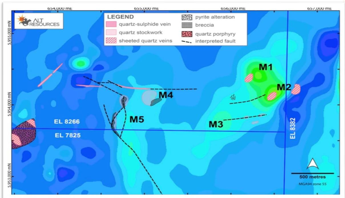
Figure 3. Horizontal slice through the magnetic model at Windy Hill, at 600m RL (between 200-300m below surface), overlain by mapped geology. The key magnetic anomalies are labelled M1-M5. The relationship between magnetic anomalism and known mineralisation features at surface is evident.
