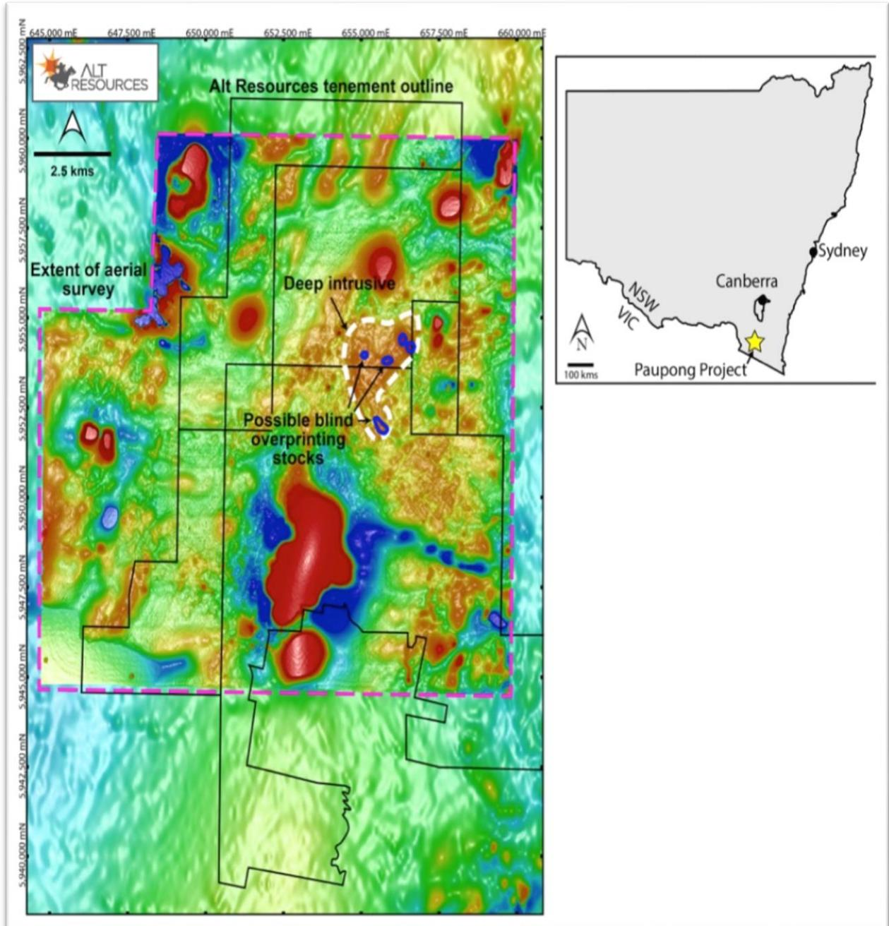
Figure 1. Aeromagnetic survey area over the Paupong Project, showing RTP magnetic response for the survey area (outlined with dashed pink line). The background image is the regional magnetic dataset (SE Lachlan Survey) RTP. Alt Resources' interpretation in the Windy Hill area shows a deep magnetic intrusion (estimated to be ~400m below surface) with later stocks rising closer to the surface (blue outlines).
