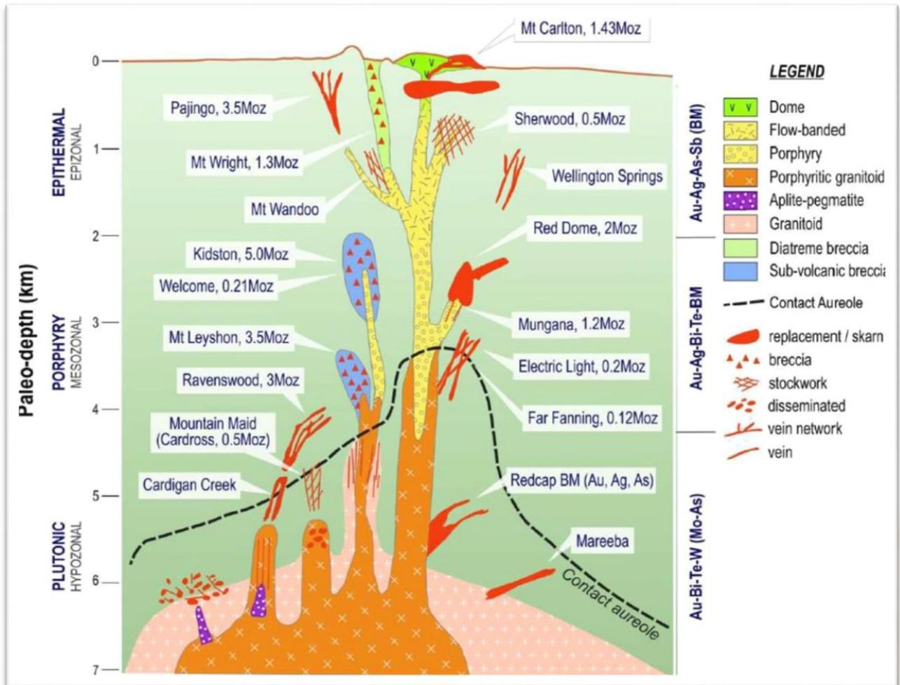
Figure 10. Conceptual model of an IRGS, with examples of the physical settings and geochemical character of various North Queensland IRG example deposits. From Morrison and Beams (2015).
