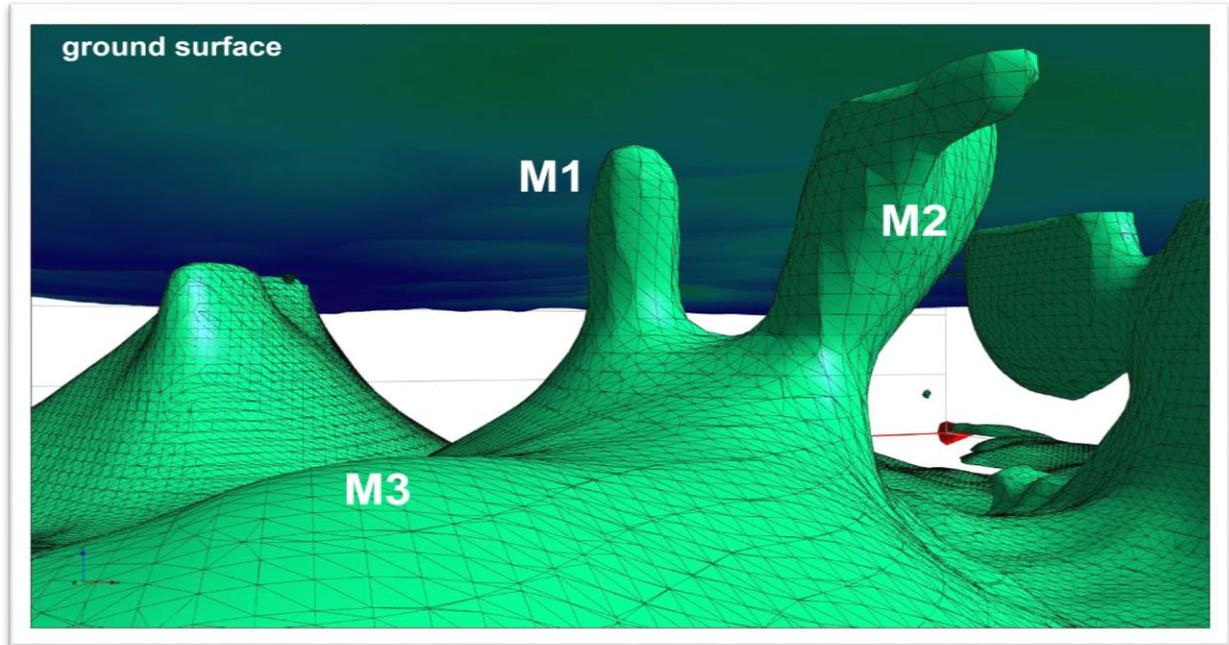
Figure 2. 3D view of the Windy Hill magnetic model. Surfaces are at 135 SI units. Key magnetic anomalies are labelled M1, M2 and M3. The view is to the North-North-East, looking up at the surface from below ground. No scale is given due to the variable distances produced from a 3D image projected onto a flat surface. The anomalies M1 and M2 are approximately 300m apart. Refer to Figure 3 for a scaled map in plan view.
