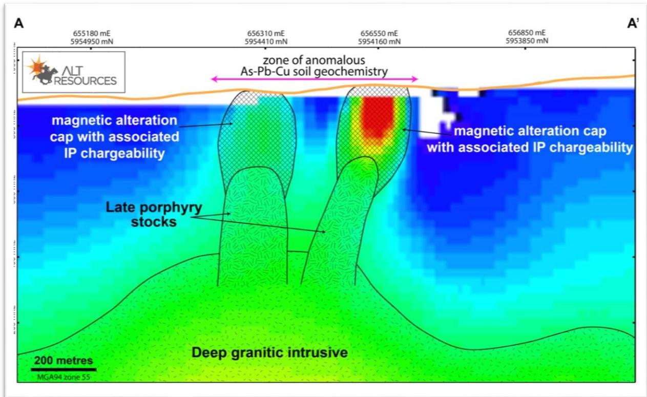
Figure 6. Cross-section of a conceptual model for the Windy Hill area. This demonstrates the relationship between a deeper intrusive body, later porphyry intrusive stocks rising to shallow levels, as well as the observed magnetic and IP responses. The base image is a vertical slice through the magnetic model, along line A-A' shown on Figure 4.
