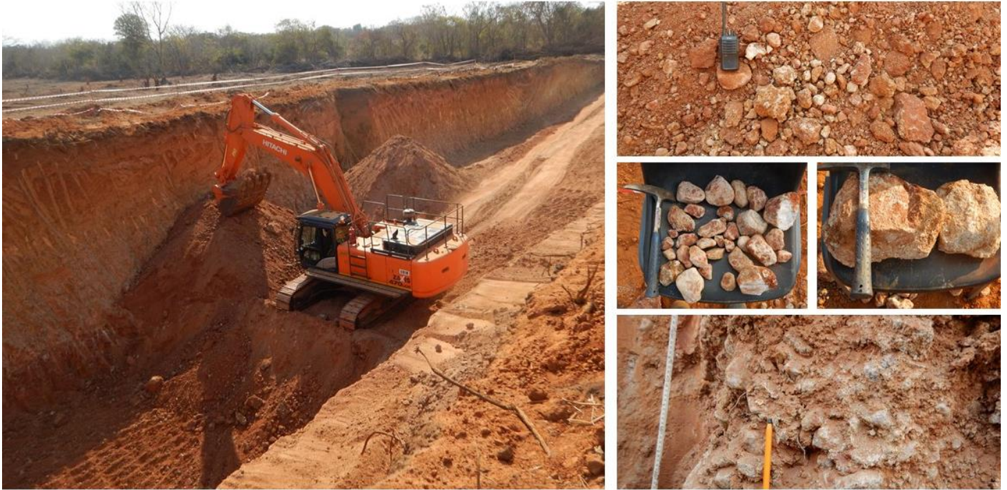
Figure 3: Pit 21. (i.) Excavation of Pit 21 down to 8m; (ii.) Gravel layer in the stock pile; (iii.) Gravel clasts of quartzite ranging from 2cm to 8cm in diameter, (iv.) Angular quartzite clasts approximately 15 cm in diameter and (v.) Gravel layer red oxidised material with white nodules and clasts
