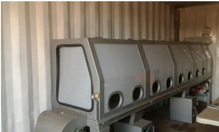
Figure 1: Mustang bulk sampling plant construction, glove-boxes & stockpiling of gravel from pit
