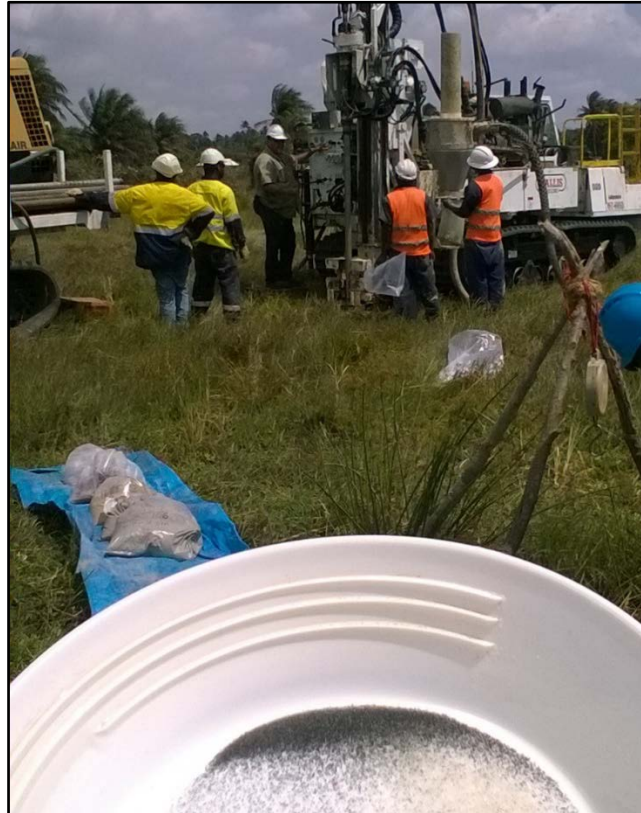
Figure 2. Aircore drilling at Fungoni with heavy mineral pan sample taken from that drill hole
