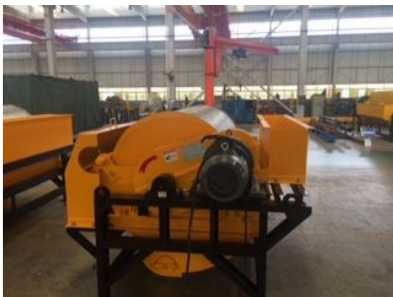
Lims Magnetic Separator equipment ready for final inspection
