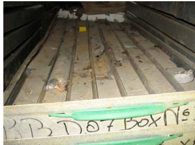
Half core from KBD 07, showing entire hole sampling
