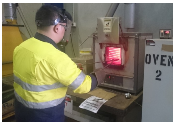
FIGURE: Bench scale roast testing.
