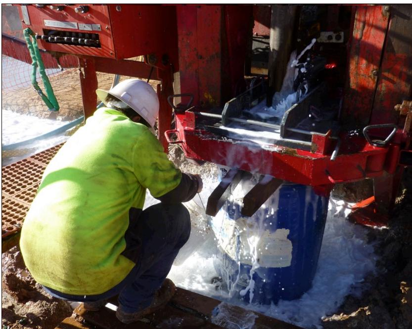
*Figure 1: Brine quality testing at test-production bore # 2, Site A*
