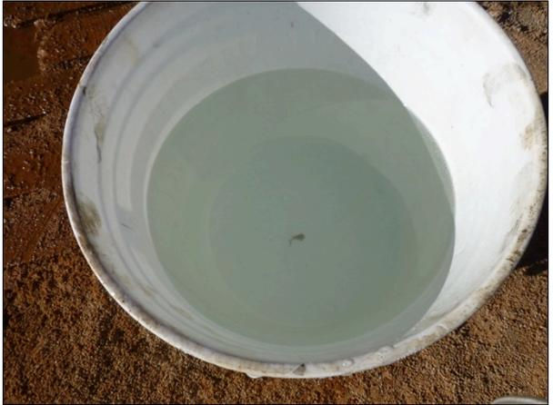
Figure 7: Clean brine flow sample after jetting
