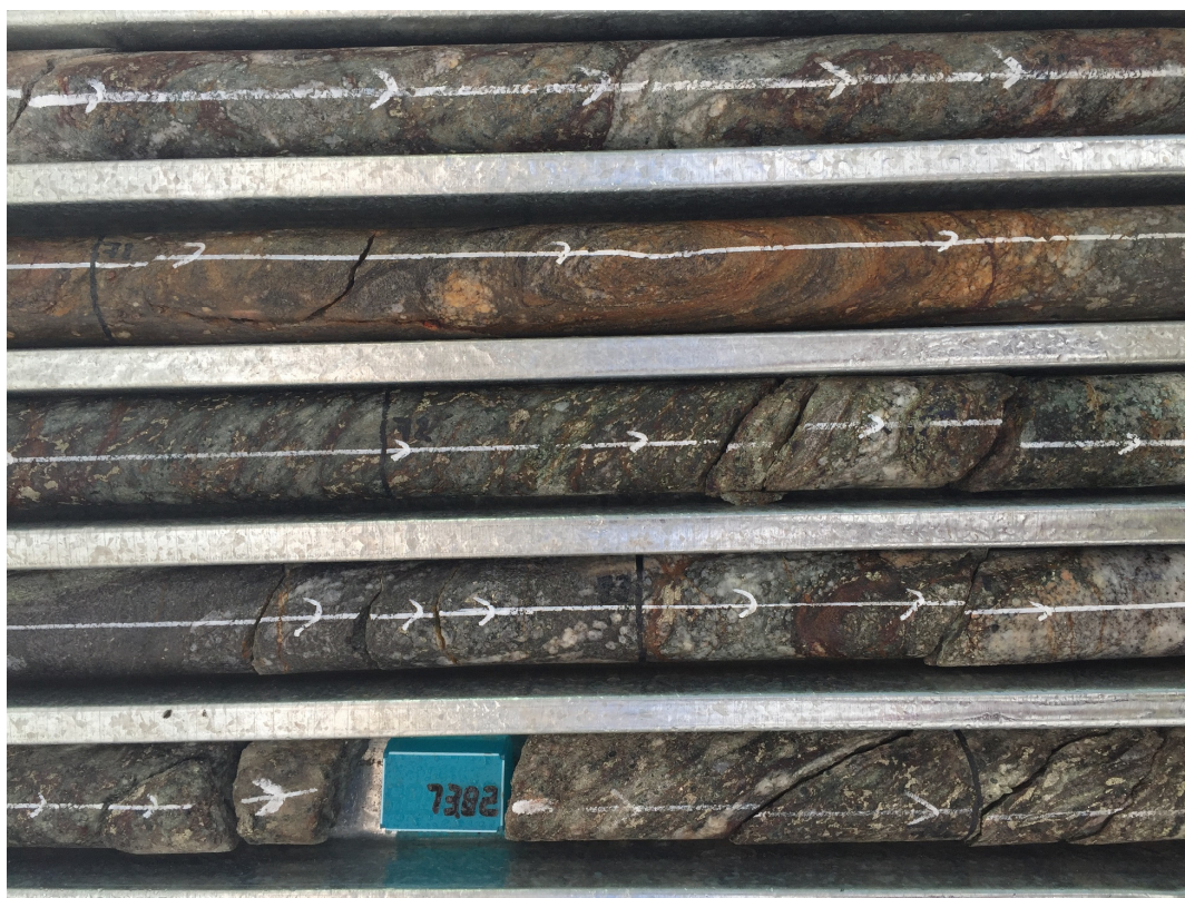
Figure 3: Highly mineralised core intersected in hole OWCD033 between 70m – 74m. Pyrite (5%-15%) is partially oxidised to haematite and limonite at this depth. Lithology is structurally complex, folded and sheared. The white line marks orientation reference line.
