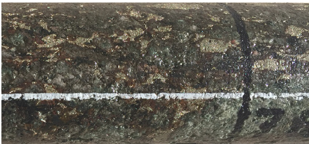
Figure 5: Highly sulphidic, blebby and net-textured sulphides associated with elevated gold-copper mineralisation, indicating suitability for EM detection.
