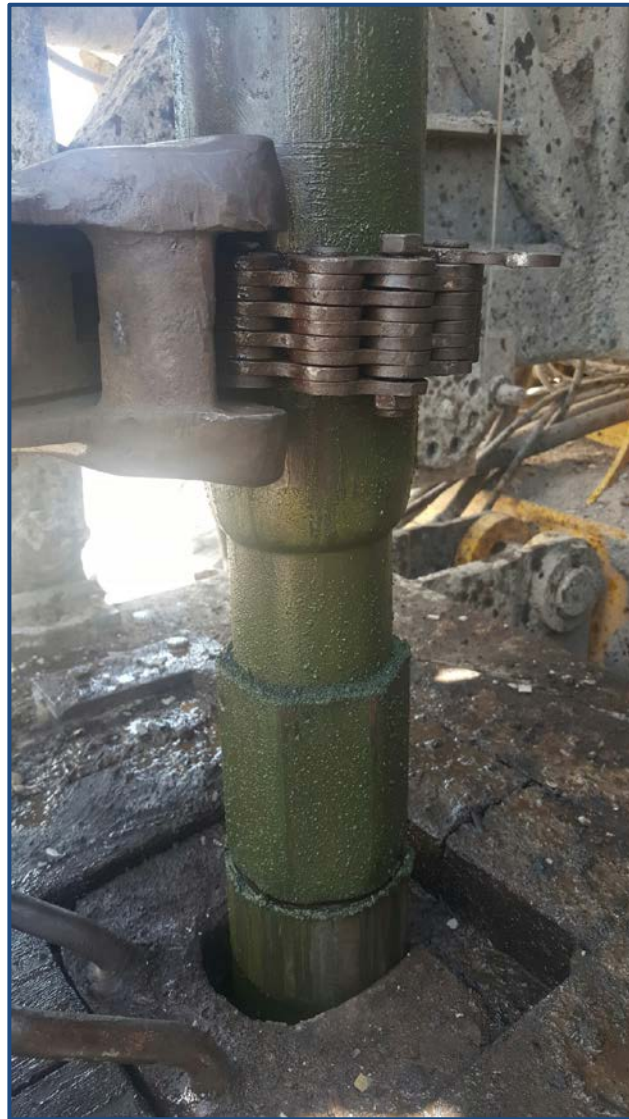
The drill string is covered in a green coloured crude oil as it is brought back to the surface
