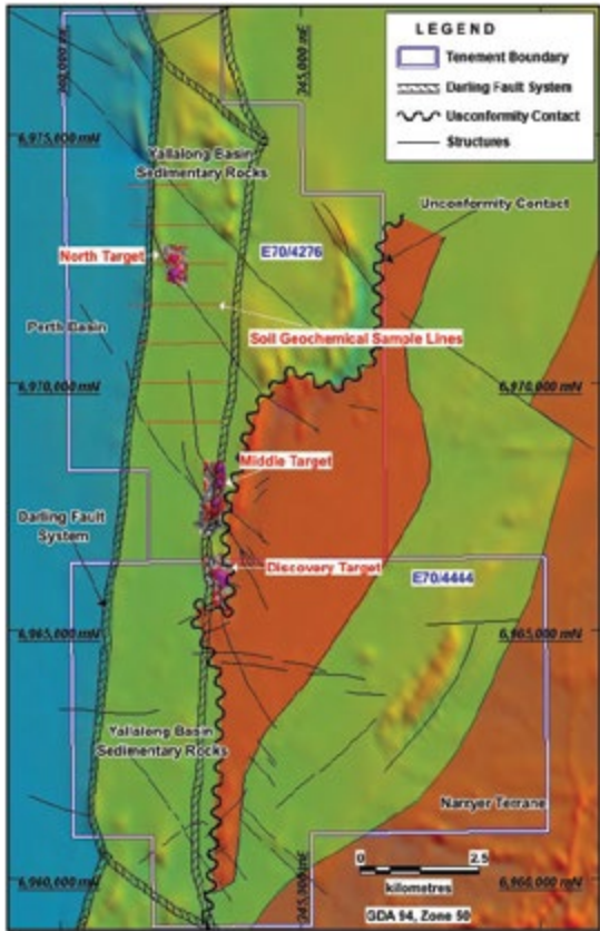
Figure 6. The Yallalong Project showing the position of the Discovery, Middle and North Targets with respect to the Darling Fault and Unconformity Contact
