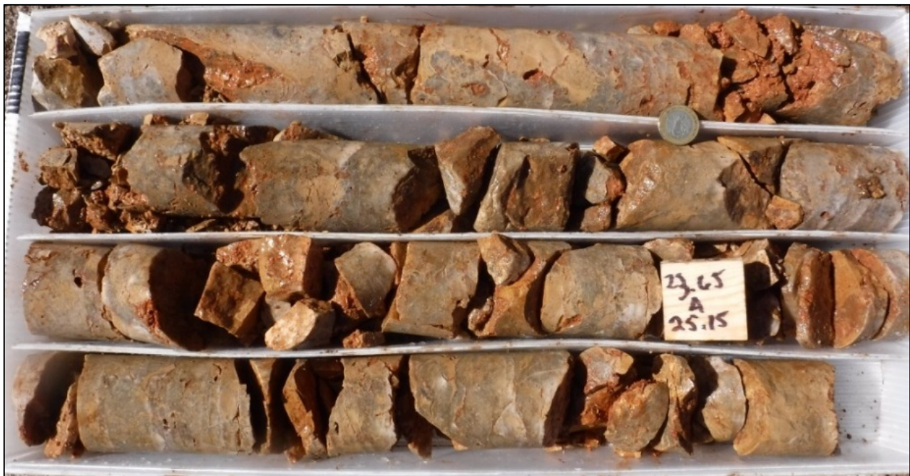
Figure 2: MDPD-012 drill core showing interval 23.65m-25.15m: 1.50m @ 5.60g/t Au
