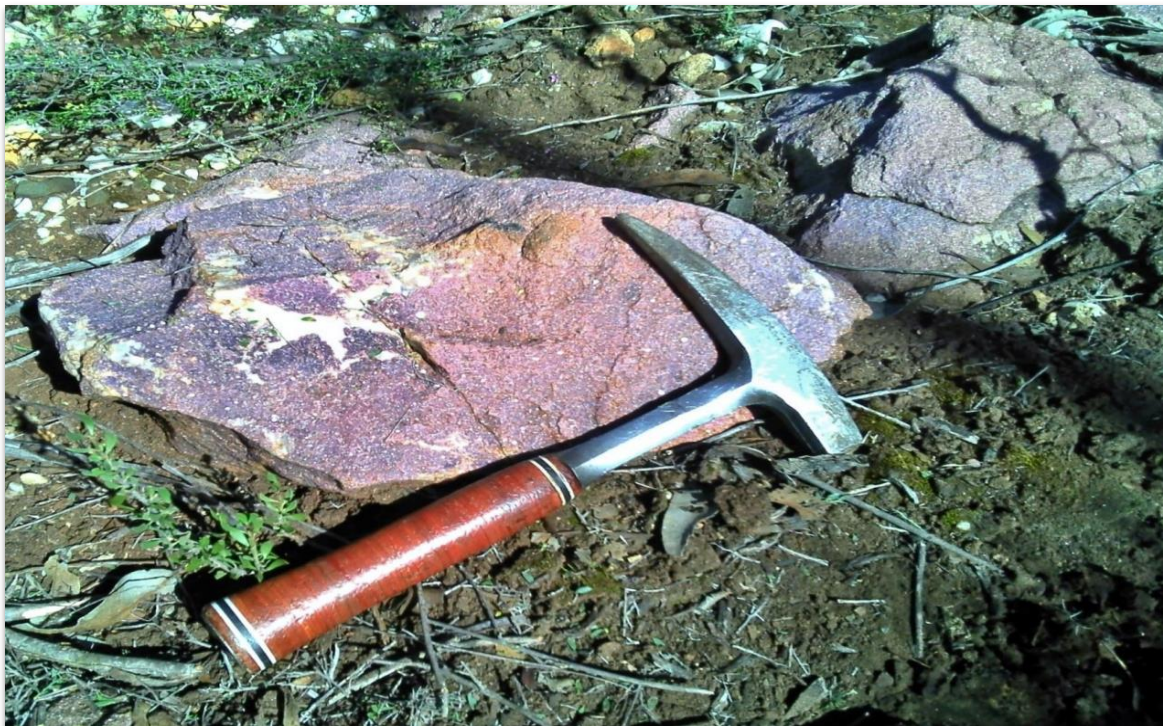
Figure 4 shows massive lepidolite in outcrop of the Boundary Pegmatite. Assay results of LJR 021, taken from this pegmatite include 3.94% \text{Li}_2\text{O} , 4.79% \text{Rb}_2\text{O} and anomalous Caesium and Tantalum (2985ppm Cs and 191ppm Ta). Massive lepidolite is a common feature of the mineralized pegmatites at Lake Johnston.
