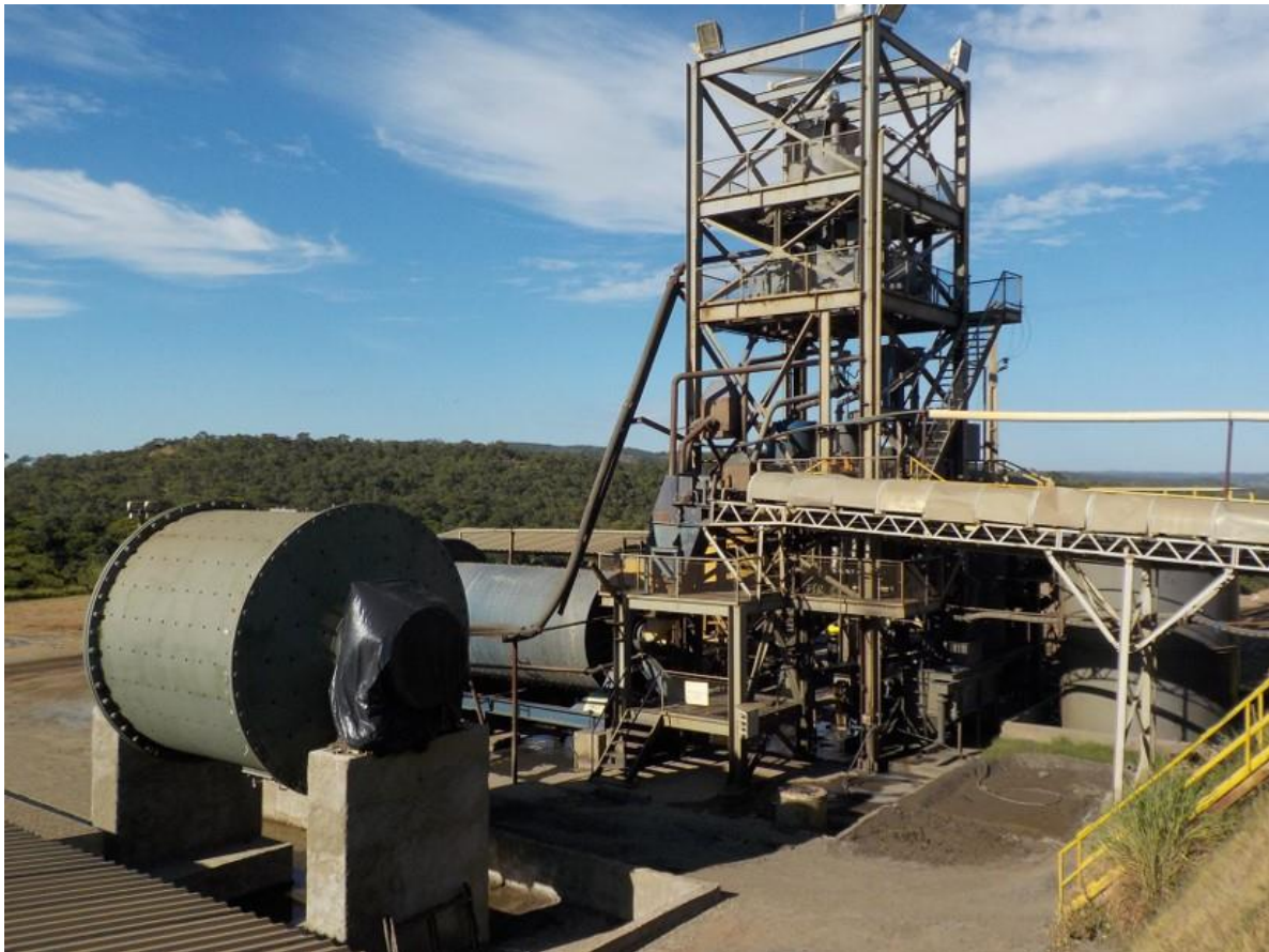
New Ball Mill in place at Premier Gold Mine (note 28-33tph mill in place behind new mill)
