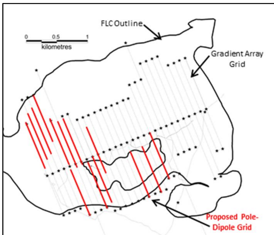
Figure 5 - IP Survey Outline. Detailing the Gradient Array Survey (black) and areas for detailed Pole-Dipole follow-up work. Reference Fig 1 for location.
