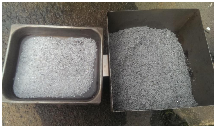
Figure 4: Left – HMS Spodumene-Tantalum Concentrate; Right – HMS Floats
