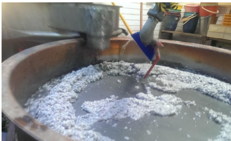
Figure 3: HMS Spodumene Concentrate (Sinks)
