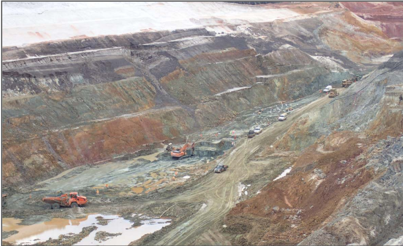
Excavator mining ore to 47.5 RL as pit floor reaches fresh rock horizon.
