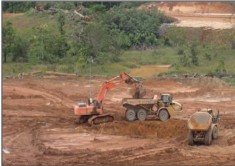
Excavator mining waste to 65 RL facing up ore.
