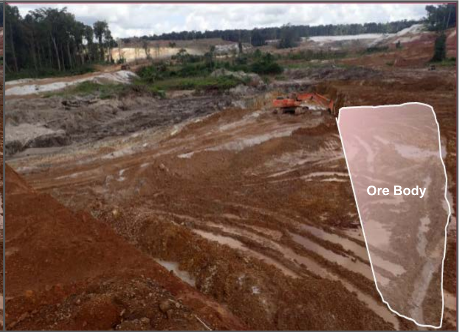
Excavator mining waste to 60 RL to face up the ore.
