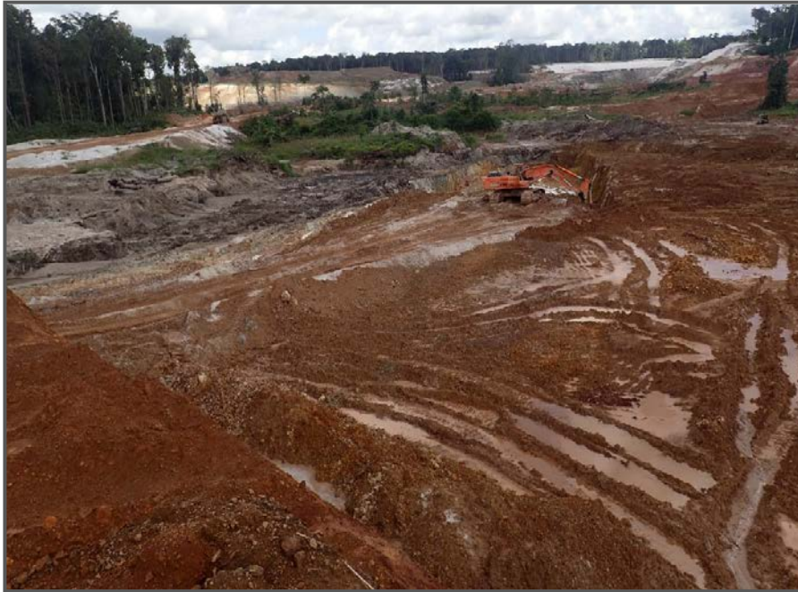
Excavator mining waste to 60 RL to face up the ore.
