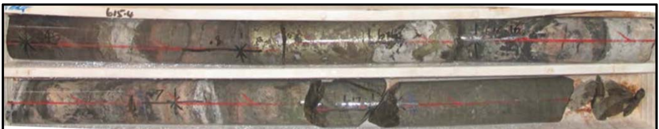
Figure 3: MHC20001 drilled in 2012 Minyari deeps brecciated chalcopyrite-quartz-calcite sulphide vein grading 0.36m at 41.55 g/t gold, 12.02% copper and 43.80 g/t silver from 615.80m (part of 16.00m at 2.50 g/t gold and 0.54% copper from 614.00m) located down dip beneath Antipa’s re-modelled Line # 6 IP target.
