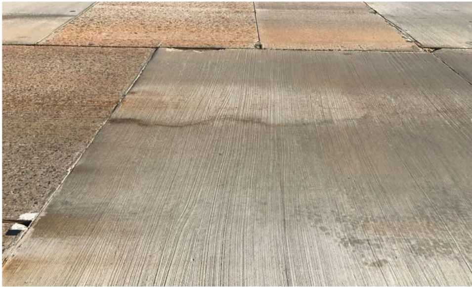
Figure 1. Control slab on I-20 Field trial showing visible crack extending across slab after 14 months
