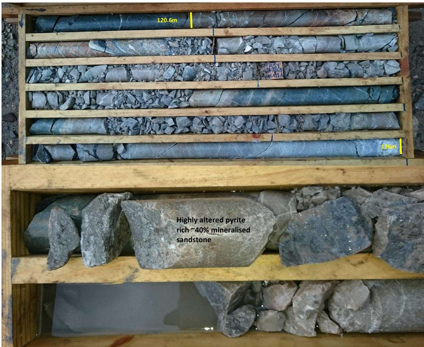
Figure 3: Intensely altered sandstone in contact with intrusive diorite. Note extensive quartz-k feldspar-pyrite alteration and in the close up how the core contains 40% pyrite.
