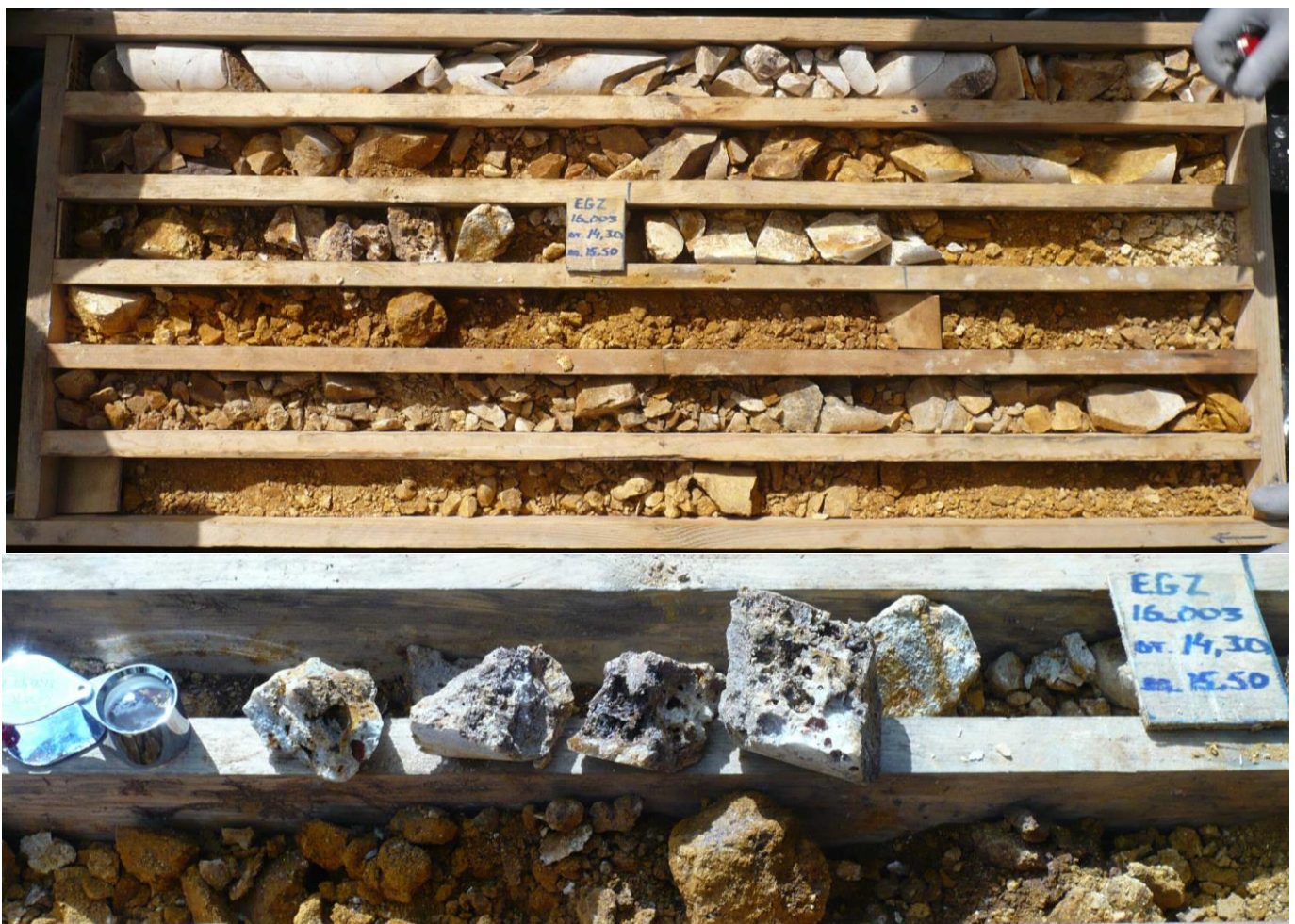
Figure 1: Mineralised zone, quartz veining showing ex-sulphide box-work (lower half) along the contact and strong orange limonite-goethite alteration (ex-sulphides) extending into the granodiorite and sandstone either side.
