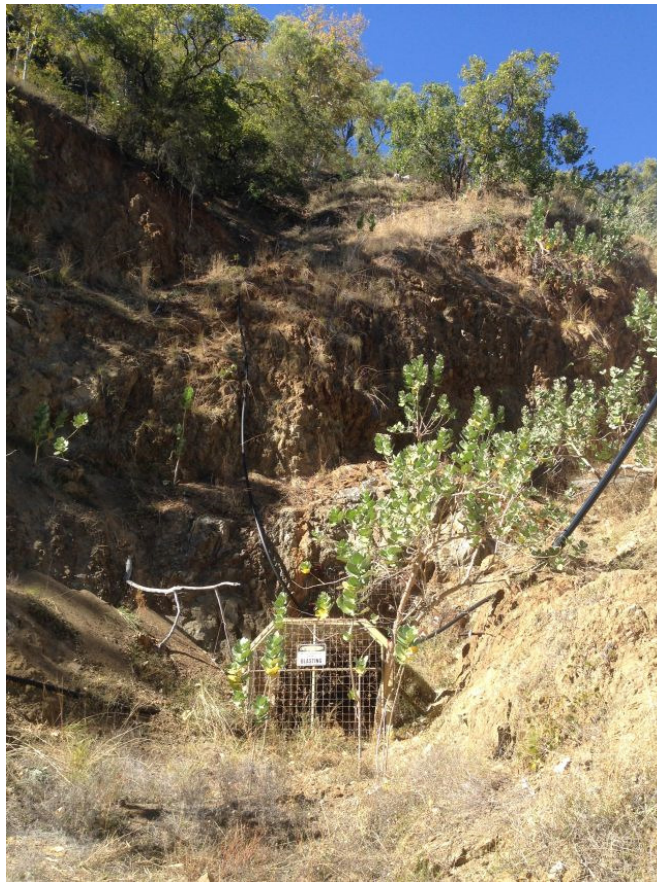
Photo 11: Flying Cow prospect showing adit and compressed air line
