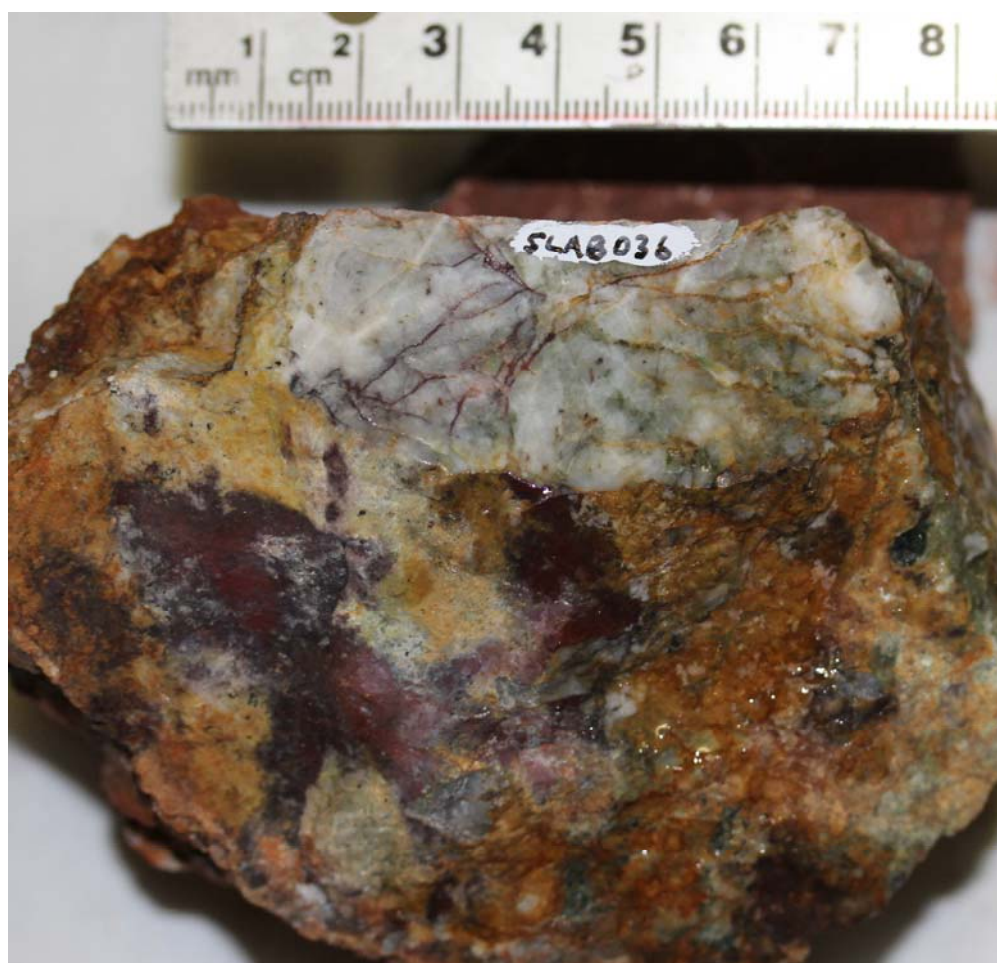
Figure 5: Surface sample from Central North of quartz breccia and saccharoidal quartz with sulphides.
