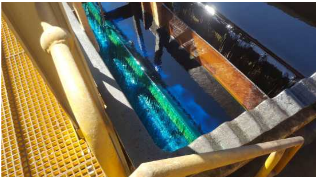
Figure 3: Electrolyte solution flowing out of the solvent extraction settlers to the electrowinning circuit
