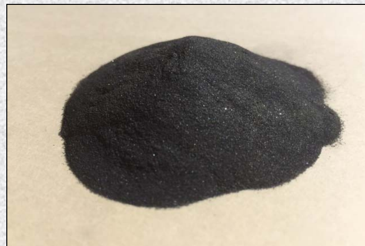
MAHUMO CONCENTRATE: 51.9% Cu & 1,300ppm Ag from test work on sulphide ores (refer announcements: 6 July 2015, 31 July 2015)
