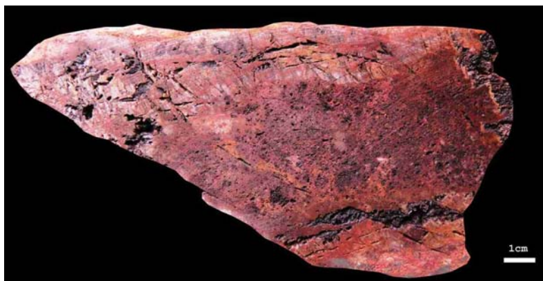
Figure 16: Quartz-hematite (after sulphide) vein. XR14247. 80.92g/t Au and 0.97% Cu.
