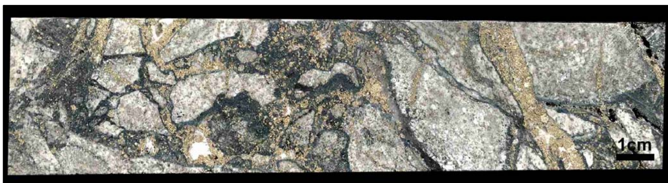
Figure 4: Tourmaline-pyrite-chalcopryite cemented breccia. KHRC267- 132m: From 2m interval grading 0.14g/t Au and 0.06% Cu.
