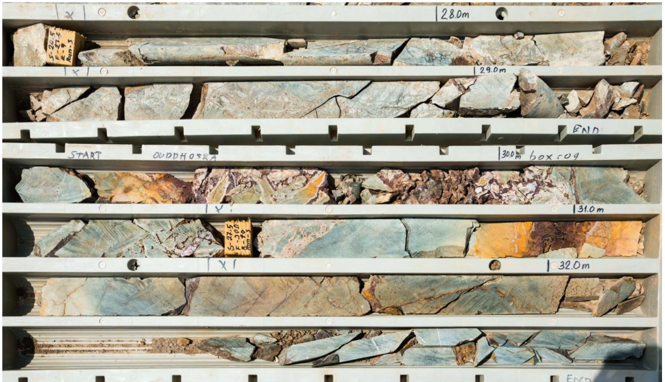
Figure 7: Epithermal Vein Infill Textures from Drill Hole OUDDH-032.
