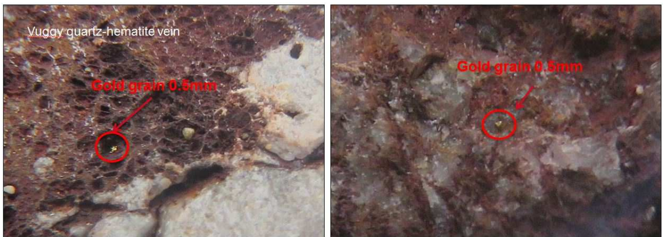
Figure 8: Vuggy hematite-quartz veins with visual coarse gold grains in drill hole OUDDH043.
