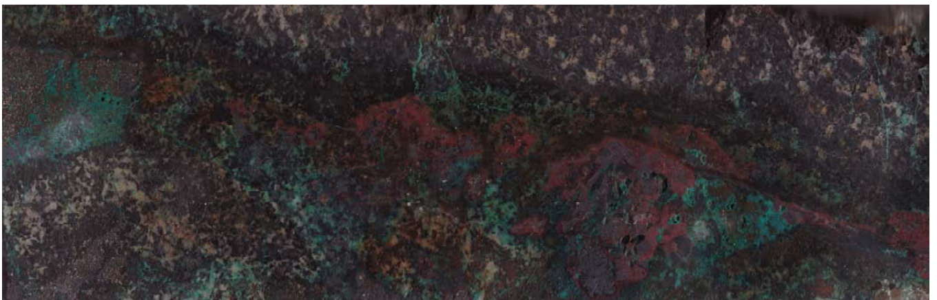
FIGURE 15: Chalcocite-chalcopyrite cemented breccia at the Breccia Pipe prospect. Ouddh036-26m: from a 2 metre intersection of 6.6% Cu.
