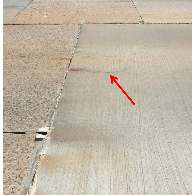
Control - Visible Crack Developing
